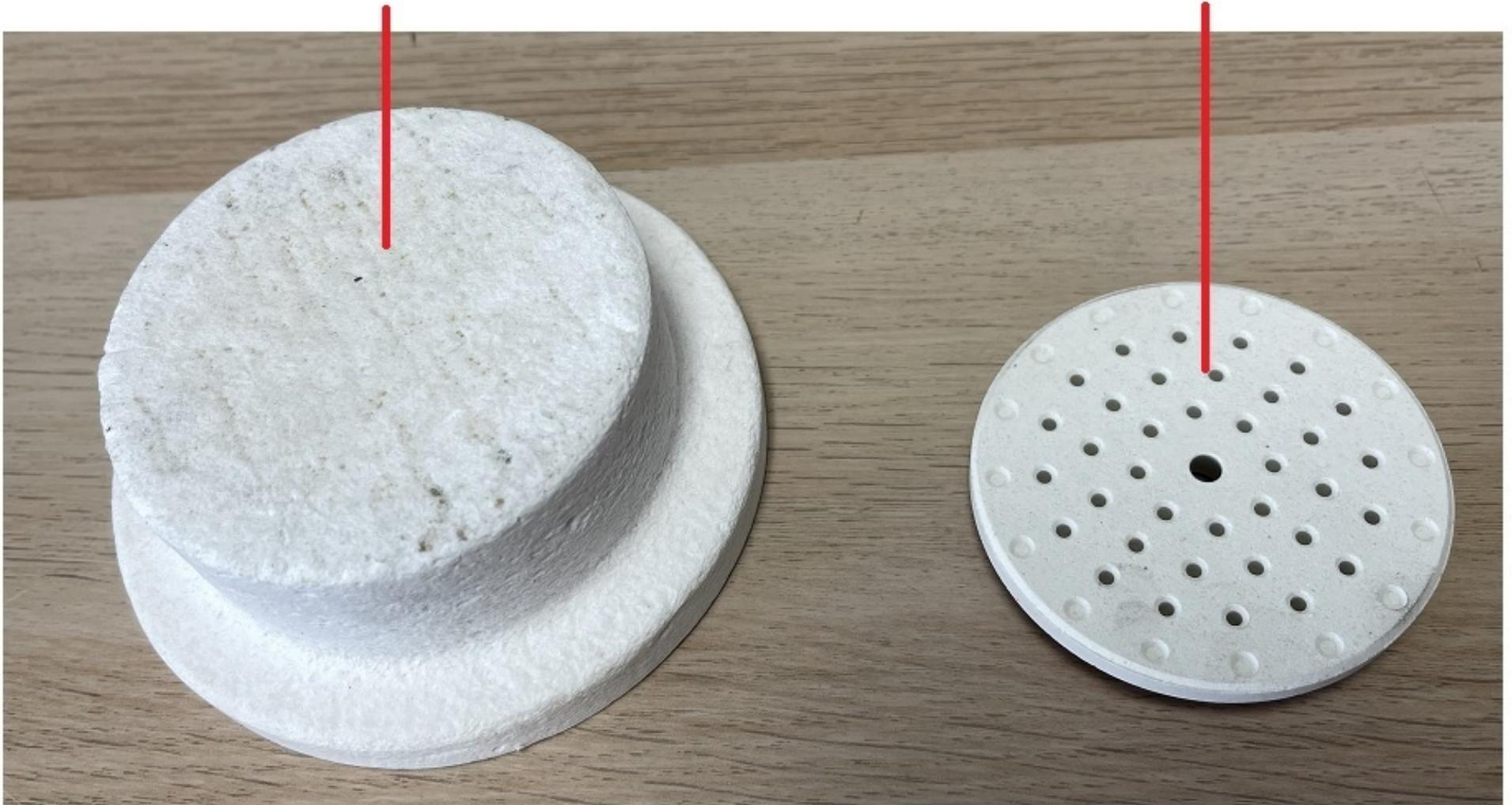
**Please keep clean or replace these items and also use the appropriate super peg for each company's material. If not It will be the cause of BLACK SPOTS when you process glaz. Furthermore, please put away these Gas Burners, Casting Machines, AC air flows etc.....tiny black particles will lead to the BLACK SPOT.**
