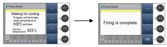
If set to a range of  $1\sim100$  °C the temperature of the final STEP, table does not decrease while the top-level firing at the end. Please set If you do not want to lower the firing table at the end of firing for the safety.
