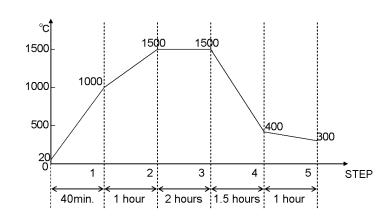
Programmed Start temperature for Zircom speed is 20 °C.
