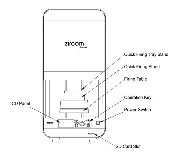
Quick Firing Tray Stand : Place to put firing tray and firing object.
